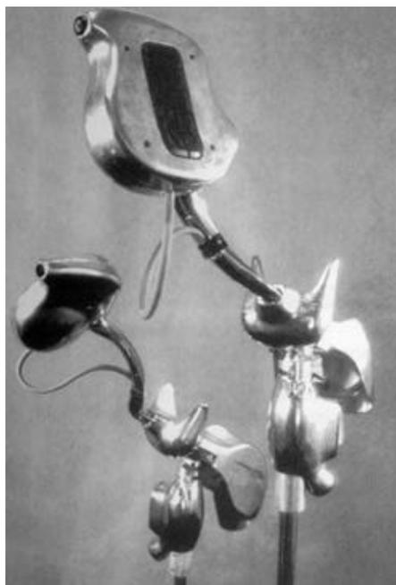
The sensor system is based in two symmetrical mechanical articulated arms with several buttons and two-foot pedals. The resulting gesture and movement data streams are transmitted over MIDI to a Macintosh computer running a program developed under MAX that processes the data and actuates over a sound synthesizer that finally outputs the sound.
