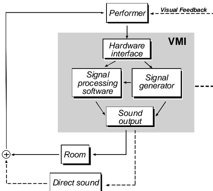
The Hardware Interface can actuate on the Signal Generator typically to vary the Pitch and Dynamics like in a traditional instrument, but it can also actuate on the Signal processing software and therefore transform all kinds of parameters.
