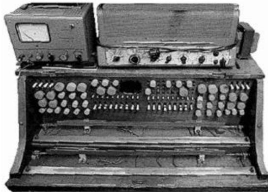
The German composer **Oskar Sala** took over the development of the Trautonium and in 1952 he built the **Mixtur-Trautonium** based on the original Trautonium but using semiconductors, and adding wire-covered catgut strings, which acted as variable resistors. According to the position at which they were pressed against the contact rail beneath them, they would control the frequencies of the electronic sound generators.
